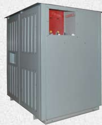
2500 KVA, Three Phase, 60 Hz ABS Certified Transformer, 6600-Volt Delta Copper Primary - 480 Volt Delta Copper Secondary With Custom Primary Take-Off, Custom Base Designed for Installation on Customer Platform and Door Mounted Heater Controls.
