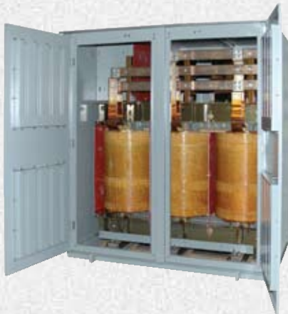
2500 KVA, Three Phase, 60 Hz ABS Certified Transformer, 6600-Volt Delta Copper Primary - 480 Volt Delta Copper Secondary With Custom Primary Take-Off, Custom Base Designed for Installation on Customer Platform and Door Mounted Heater Controls.
